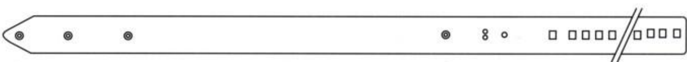
ISHIKAWA RAPIER TAPE 1001 WIDTH 30 mm. THICKNESS 2.5mm RIGHT
